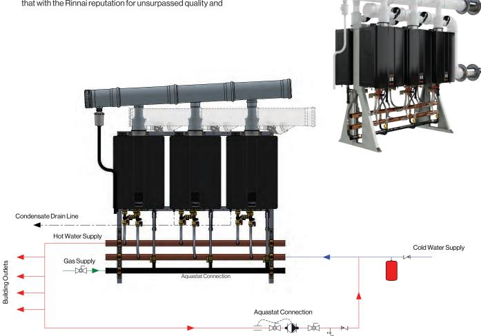
Simulated TRS with recirculation installation shown
