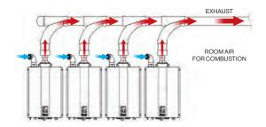
\*HE+ Series tankless water heaters must use concentric venting with a metal exhaust pipe. Refer to the Installation and Operation Manual supplied with the HE+ Tankless Water Heater for venting options
